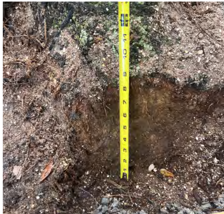
Image 16 This show the 9-inch diameter root that was cut to accommodate the curb. The cut was only 12 inches from the tree making the tree less stable.
